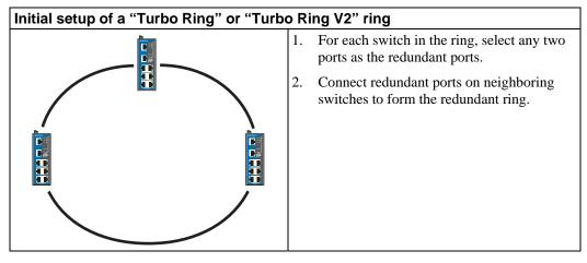
The user does not need to configure any of the switches as the master to use Turbo Ring or Turbo Ring V2. If none of the switches in the ring is configured as the master, then the protocol will automatically assign master status to one of the switches. In fact, the master is only used to identify which segment in the redundant ring acts as the backup path. In the following subsections, we explain how the redundant path is selected for rings configured for Turbo Ring, and Turbo Ring V2.
